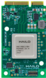
Figure 3: Hailo-8 mPCIe board
